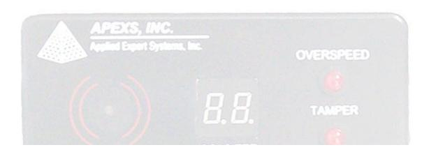
(7) To calibrate\*, press Mode to display 5 and press the Enter switch, the letters CA will be displayed. Drive the vehicle at 40Kph or 40Mph while another person doing the calibration watches the vehicle speedometer. When the speedometer indicates 40Kph or 40Mph the red Enter button is pressed a "Beep" will be heard. This completes the calibration for high speed range monitoring.
